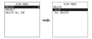
To display the delete operation menu, select DELETE in the Disk menu and press the ⇒ (OUT) button. In the delete operation menu, select CLIP or ALL DELETE and press the SET button to delete individual clips or all clips.
